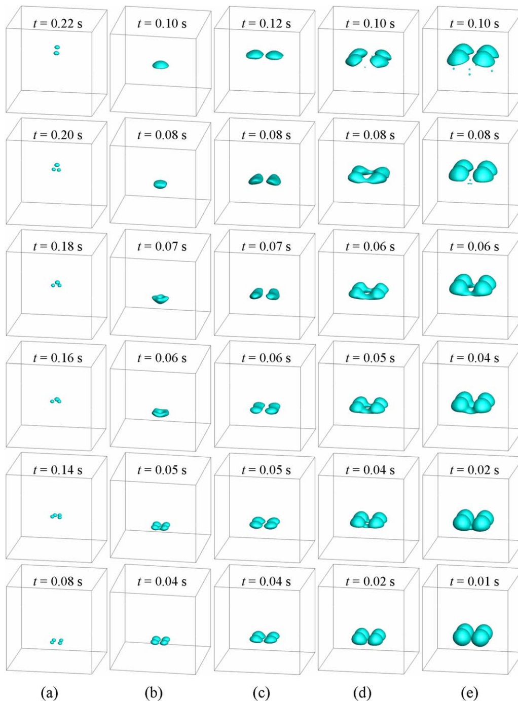
Figure 8. Coalescence processes of four bubbles with square arrangement.
