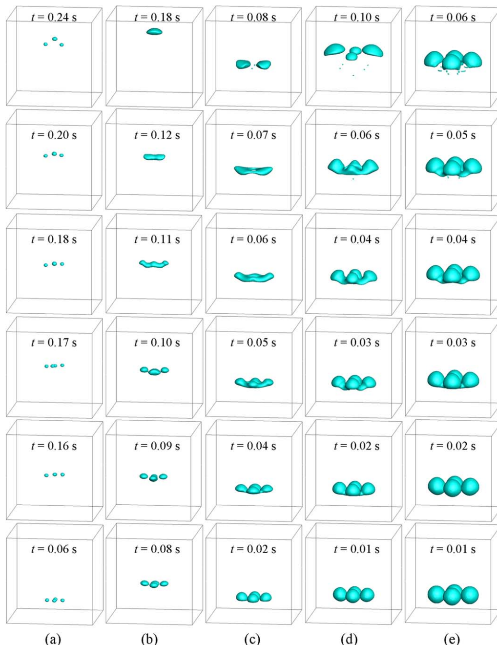
Figure 7. Coalescence processes of four bubbles with rhombic arrangement.
